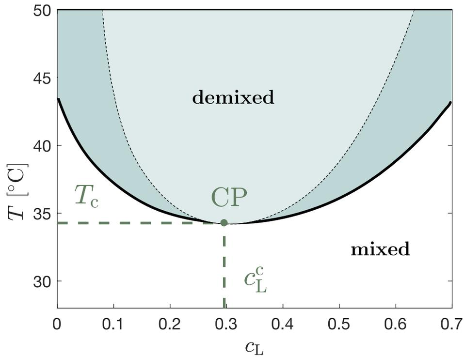
**Extended Data Fig. 8 | Phase diagram of a water–2,6-lutidine liquid mixture.** The binary solution of water and 2,6-lutidine possesses two distinct phases given by the binodal (black line) and spinodal line (black dotted line) separating mixed
