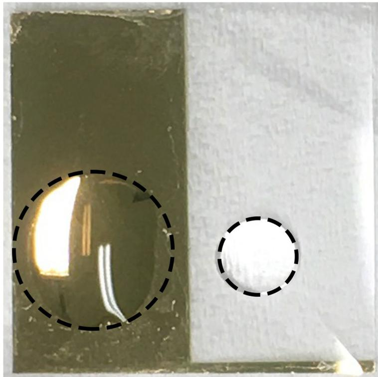
**Extended Data Fig. 9 | Effect of the treatment with different self-assembled monolayers (SAM).** Side and top view of a cover glass slide half of which has been sputtered with a 30 nm gold layer (left half). The treatment with hydrophilic
