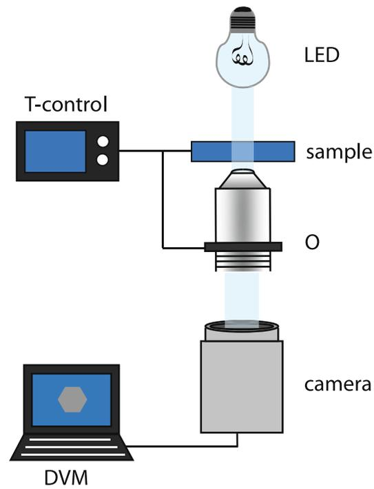
**Extended Data Fig. 2 | Schematic of the experimental setup for digital video microscopy.** Homemade version of an inverted brightfield microscope consisting of a white light (LED) illuminating the sample from above, which is temperature-stabilized by using a two-stage temperature controller at the
