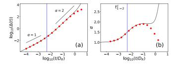
FIG. 3. Mean-square displacement (a), scaling exponent  $\alpha$  (b), and crossing time  $t_{1\rightarrow 2}^{c}$  for an underdamped active particle in a random single mode motility field. The parameters  $v_0 = 20\sqrt{DD_R}$  and  $\zeta = 20\sqrt{DD_R}$ ,  $L = 100\sqrt{D/D_R}$  feature the initial diffusive behavior and the ballistic behavior.
