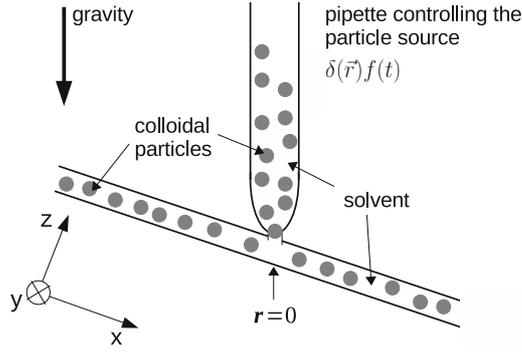
**Fig. 1.** Injection of colloidal particles into a tilted, flowing suspension.
