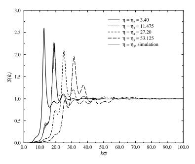
**Figure 6.** The structure factor S(k) at the magic values of the packing fraction  $\eta_m$ , for m = 2, 3, 4 and 5.
