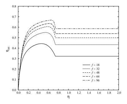
**Figure 8.** The effective hard-sphere packing fraction  $\eta_{HS}$  obtained by the procedure described in section 4 as a function of the true packing fraction  $\eta$  for five different values of the functionality f.
