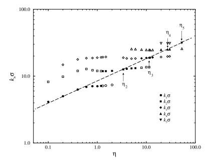
**Figure 7.** A log–log plot of the positions of the various peaks of S(k) against the packing fraction  $\eta$ . The filled symbols indicate the highest peak (see the text). The arrows indicate the locations of the magic packing fractions  $\eta_m$  and the dashed straight line has slope 1/3.
