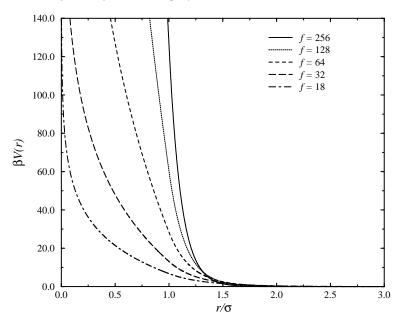
**Figure 1.** The pair potential given by equation (1) for f = 18, 32, 64, 128 and 256 as a function of the centre-to-centre separation r.
