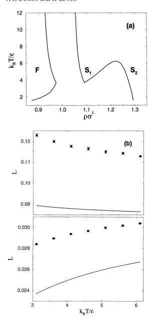
**Figure 4.** The square-well-barrier system with well and barrier width  $\delta/\sigma=0.06$ , with the same format as figure 2. (a) The predicted phase diagram, exhibiting stable isostructural (fcc) solid-solid coexistence. (b) The Lindemann ratio, exhibiting anomalous T-dependence at density  $\rho\sigma^3=1.092$  (upper panel).
