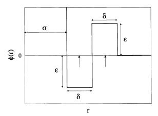
**Figure 1.** The model pair potential, consisting of a hard core of range  $\sigma$ , a square well, and a square barrier of equal width  $\delta$  and depth/height  $\varepsilon$ . The arrows on the horizontal axis indicate nearest-neighbour distances for densities corresponding to figures 2–4(b).
